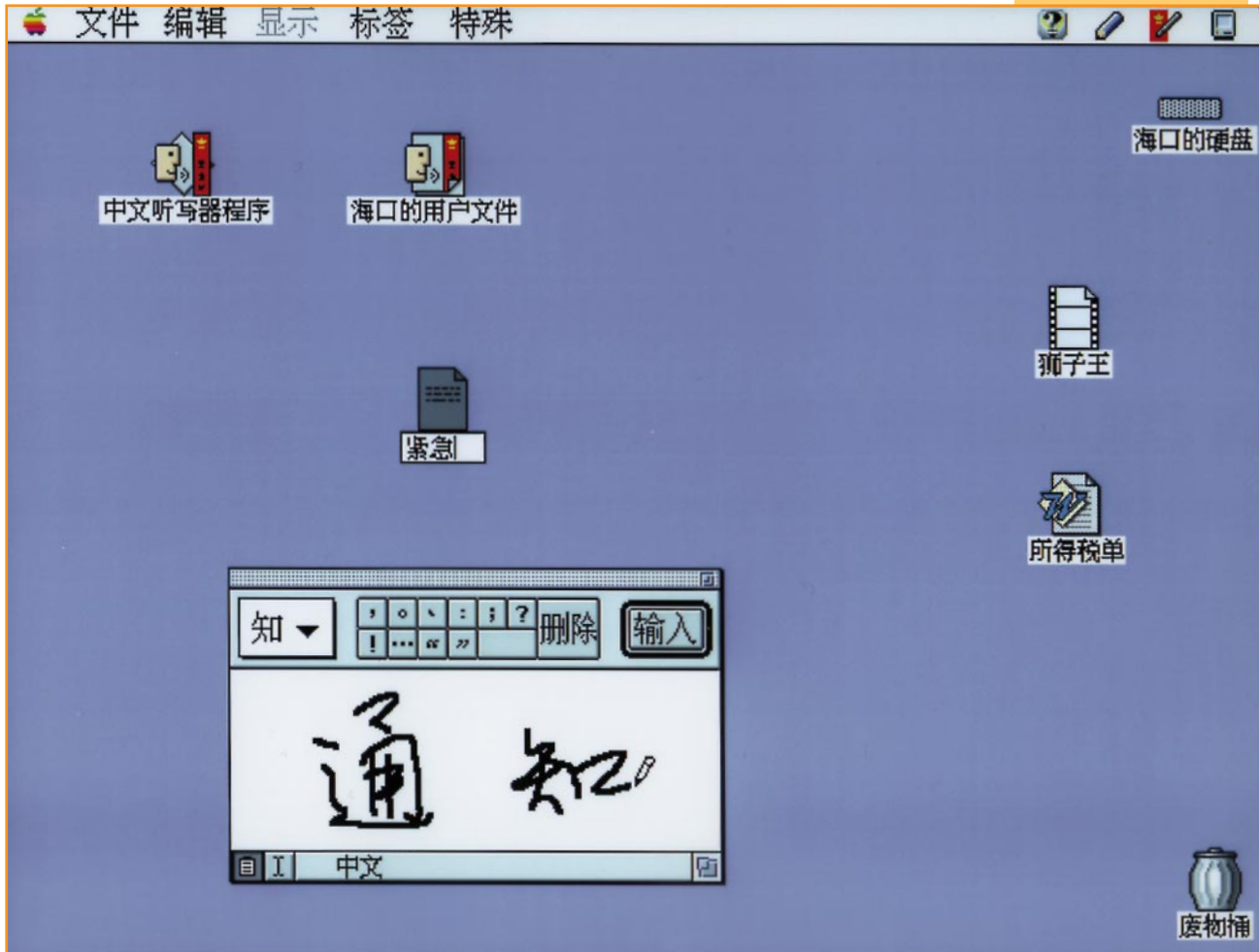
Figure 4 A Chinese name for a folder is created by handwriting. With the Chinese Input Suite users can input Chinese characters directly into all documents or text fields in the Macintosh Finder.
