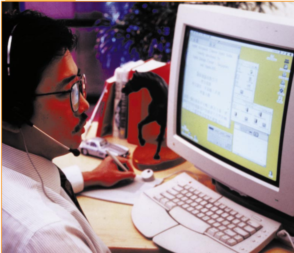
Figure 3 The Apple Advanced Chinese Input Suite integrates a microphone, a tablet and several software components into a comprehensive human interface solution for Chinese text entry.
